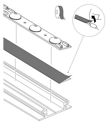
Place the module completely flat on the profile.
